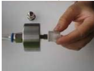
Screw the Handpiece Tip onto O-Ring
